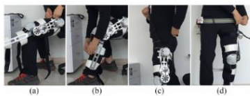
Fig. 7. Procedure of customizable braces as the mechanical interface attachment. (a) The unprocessed thermoplastic is machined to form raw part of universal shape. (b) Raw part is heated and applied on user's leg with the mechanical frame. (c) Raw part cools down and forms customized brace. (d) Precise fit with the user's limb.
